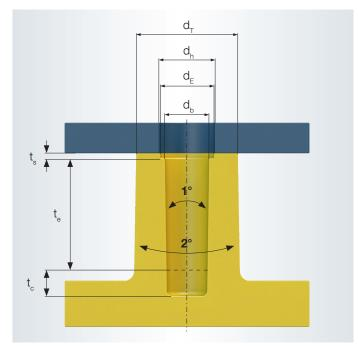
Nominal diameter of the screw: d<sub>1</sub> Counterbore diameter: d<sub>E</sub> = d<sub>1</sub> × 1.05 Hole diameter: d<sub>b</sub> = 0.85 x d<sub>1</sub>  $\pm$  0.05 mm Installation depth: t<sub>e</sub> = 2 x d<sub>1</sub> or deeper  $d_{T} = external boss \emptyset$  $d_{h} = clearance hole \emptyset$
