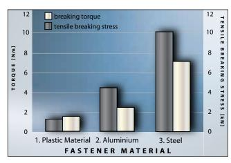
Comparison of the breaking torque and the tensile
