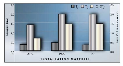
Screw: EJOT DELTA PT® P 50x25 - Installation depth: 10 mm - Hole diameter: 4 mm
