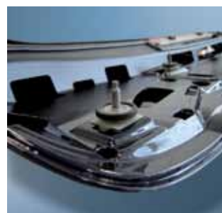
Rear spoiler fastening with the 3D adjustment mechanism
