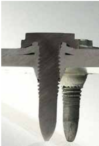
Application example: Aluminium sheet on extruded aluminium profile
