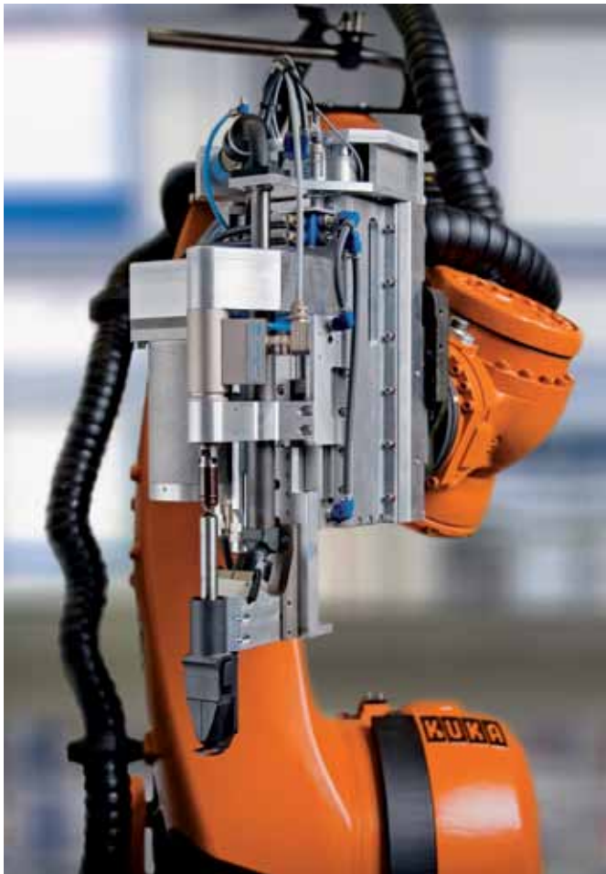
Robot-aided fastening system by Weber Schraubautomaten
