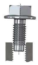
The round shaped MAThreads® are guided into contact and start to cam over the female thread.
